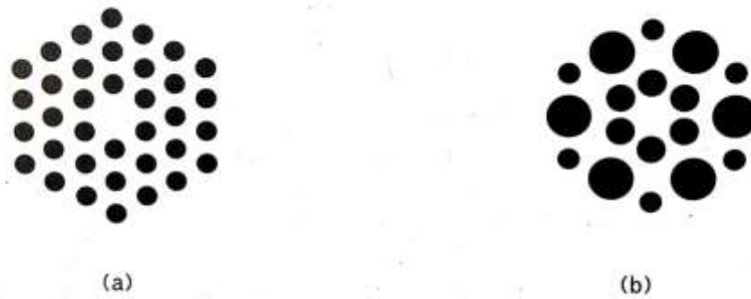
Fig: Two index guided photonic crystal fibers .The dark areas are air holes and white areas are silica.
